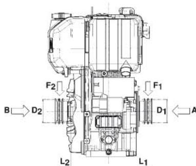
$$D_2 \text{ (mm)} \geq 740 [90 + L_2 \text{ (mm)}] \frac{N \text{ (kW)}}{n \text{ (RPM)}}$$
